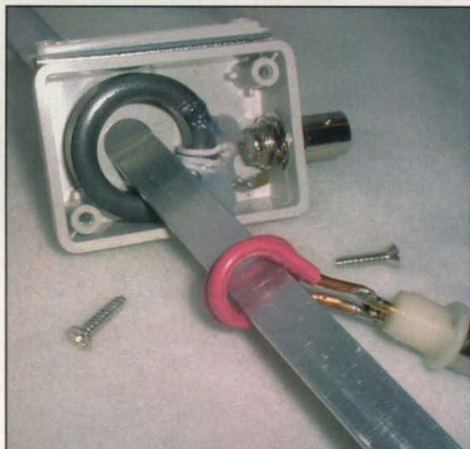
Photo E— Workings of the magnetic coupler and my 6-meter version.
