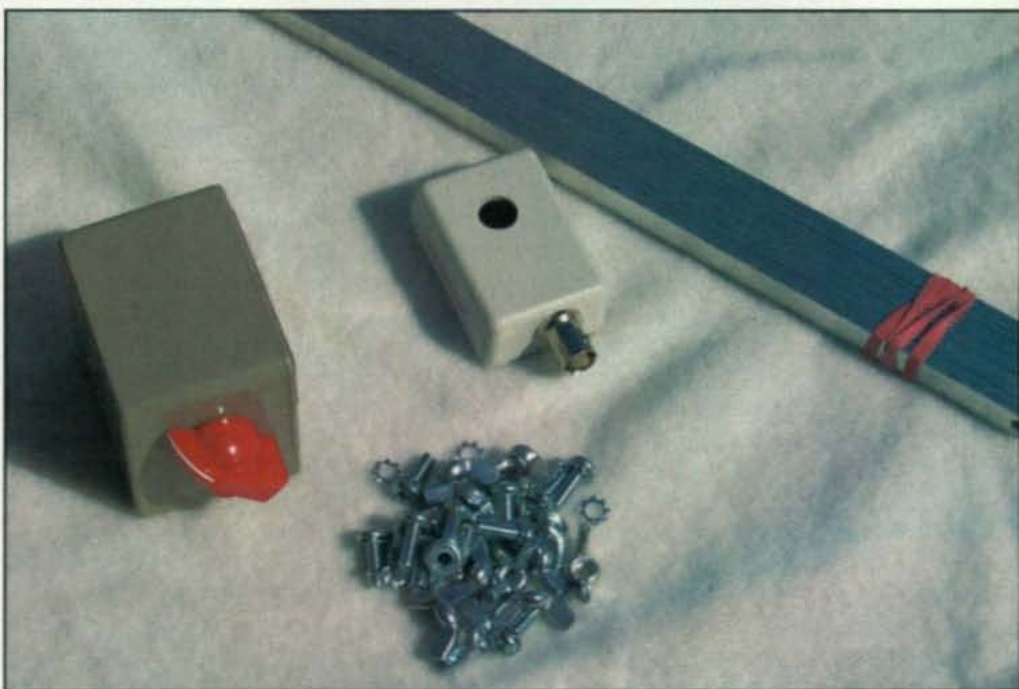
Photo C— Close-up of the tuning unit and coupler.
